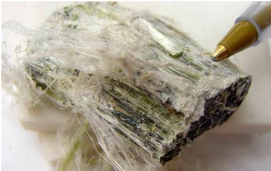
Figure 8.10 Chrysotile, Exhibits a Splintery Fracture. Image is used under a CC BY: Attribution license.
