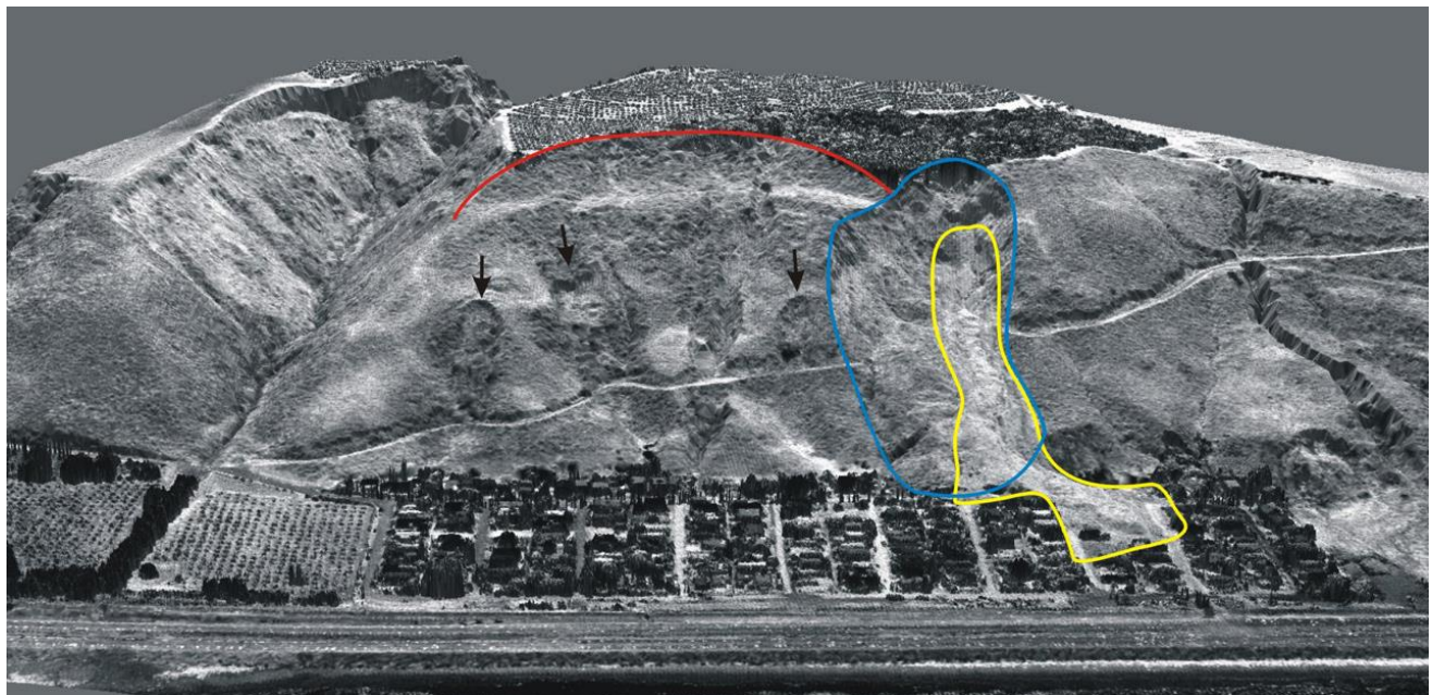
Figure 12.63 Landslides of La Conchita, Outlined in Blue is the 1995 Slide, Yellow is the 2005 Slide. Image courtesy of Airborne 1 Corporation, El Segundo, California is in the public domain.
